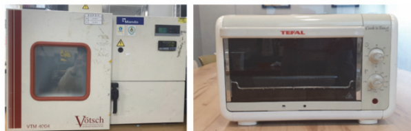
Fig. 9 Temperature chamber(left) small oven(right)
