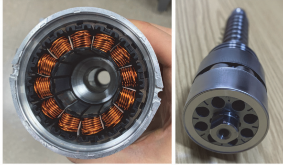
Fig. 8 SPMSM motor stator (left) rotor (right)
