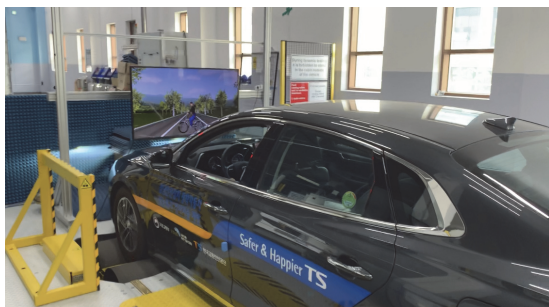
Fig. 1 VILS environment for ADAS inspection
