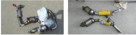
Fig. 4 Catalytic converter sample (Model 2, Model 3)
