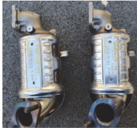
Fig. 9 Prototype catalytic converter for SULEV30 (Model 4)
