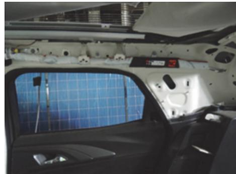
Fig. 14 Installed curtain airbag at body
