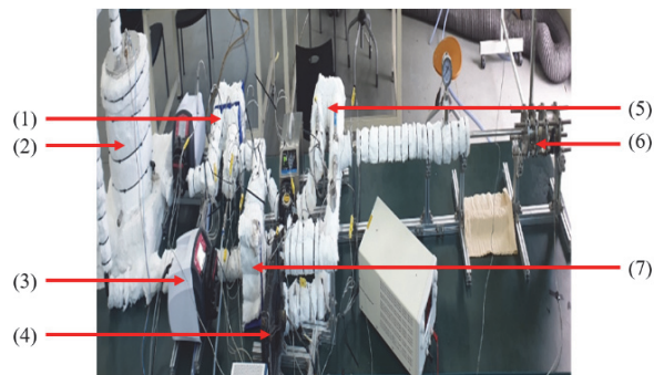
Fig. 3 Actual vortex tube experimental unit - (1) : Plate heat exchanger 1, (2) : Heat device, (3) : Water pump, (4) : Radiator and cooling fan, (5) : Plate heat exchanger 3, (6) : Vortex tube, (7) : Plate heat exchanger 2
