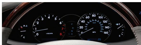
Fig. 18 Digital driven analogue type instrument cluster, 2010 Toyota Avalon
