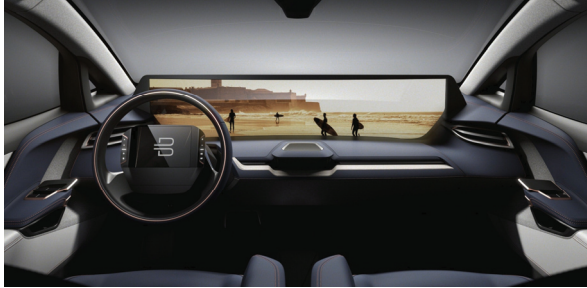
Fig. 10 Horizontal type Instrument panel of 2019 Byton EV Model
