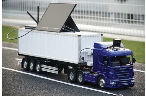
Fig. 4 1/14 Scale autonomous truck consisting of lidar and camera sensors for platooning experiments
