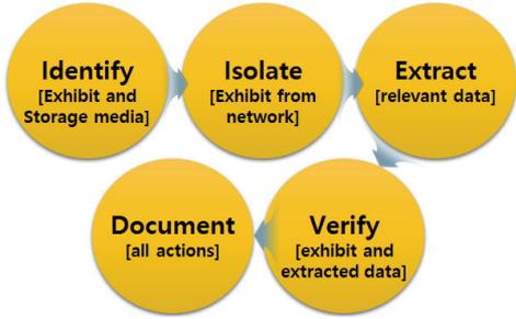
Fig. 1 Process of mobile forensic data acquisition
