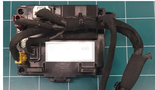
Fig. 2 Drive video record system in K7
