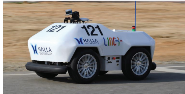
Fig. 1 Autonomous delivery platform based on ERP-42
