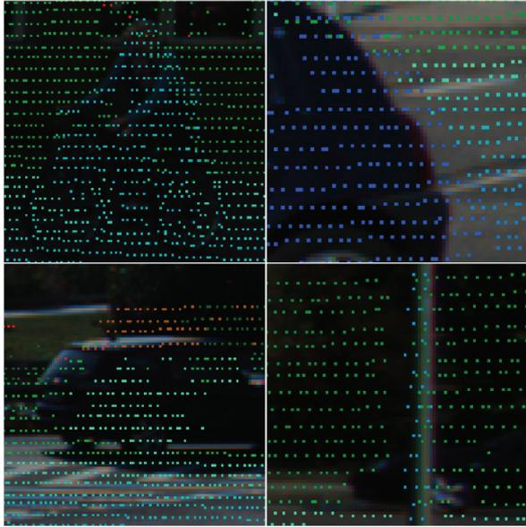
Fig. 3 Occlusion problem of the projected point cloud
