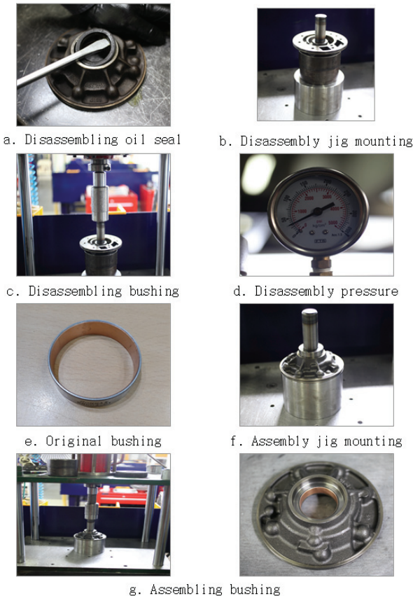
Photo. 4 Bushing assembly process
