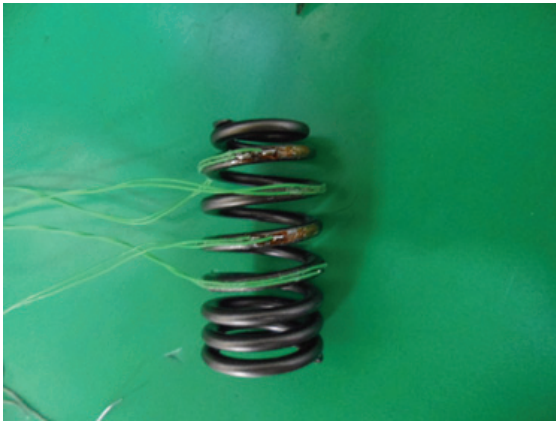
Fig. 6 Photo of strain gauges attached to the beehive spring
