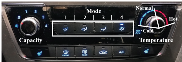
Fig. 3 Air conditioning system of simulator
