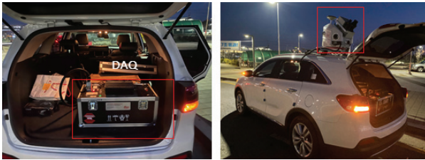
Fig. 1 Mobile mapping system calibration setup
