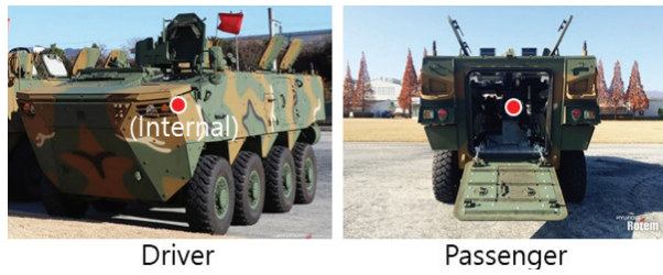
Fig. 10 Sound measuring points of the wheeled armored vehicle
