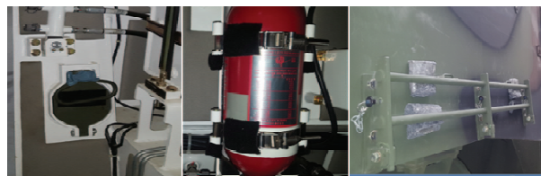
Fig. 11 Fastening for elimination of Squeak and Rattle
