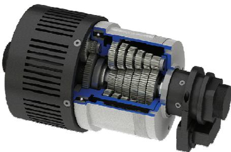
Fig. 1 In-wheel motor-transmission assembly for test vehicle
