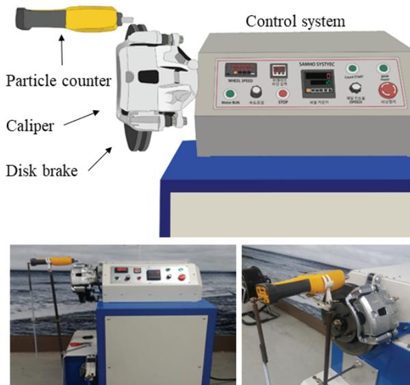
Fig. 1 Brake dust measuring system with a particle counter
