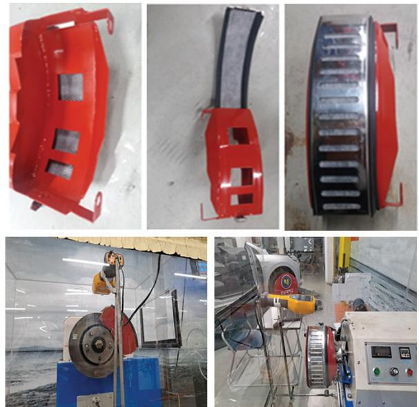
Fig. 4 Measurement method of dust scattering with the dust collector
