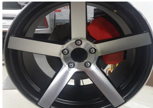
Fig. 11 A caliper integrated self-designed dust collector in an automotive disk brake system
