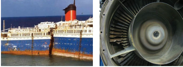
Photo. 1 Fatigue failure of a large ship(left) and aircraft engine turbine(right) under random vibration
