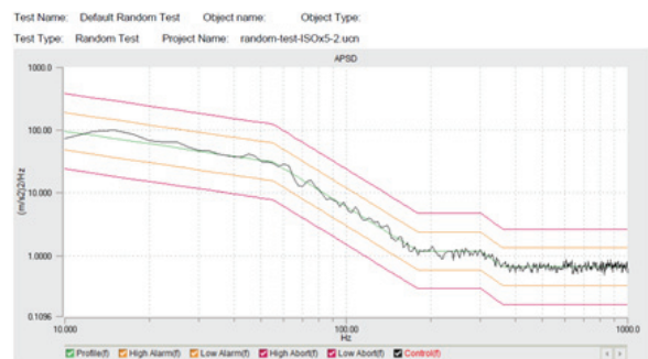
Fig. 9 Random fatigue test input acceleration PSD(ISO 16750-3 x5)
