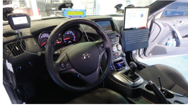
Fig. 3 Installation of VBOX 3i system in test car
