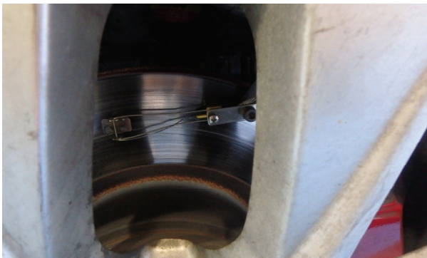
Fig. 7 Installation of thermocouple in test car
