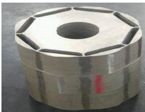
Fig. 10 Manufactured rotor and SBW motor
