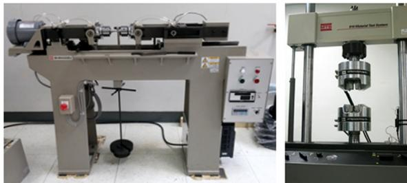
Fig. 4 H-7 rotary bending fatigue tester and MTS 810 universal tester
