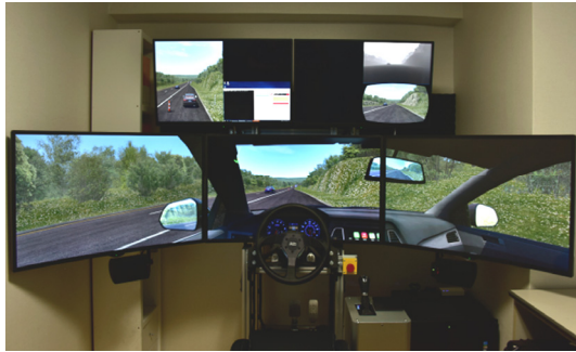
Photo. 1 Simulator for tuning and validating the P-EPS performance
