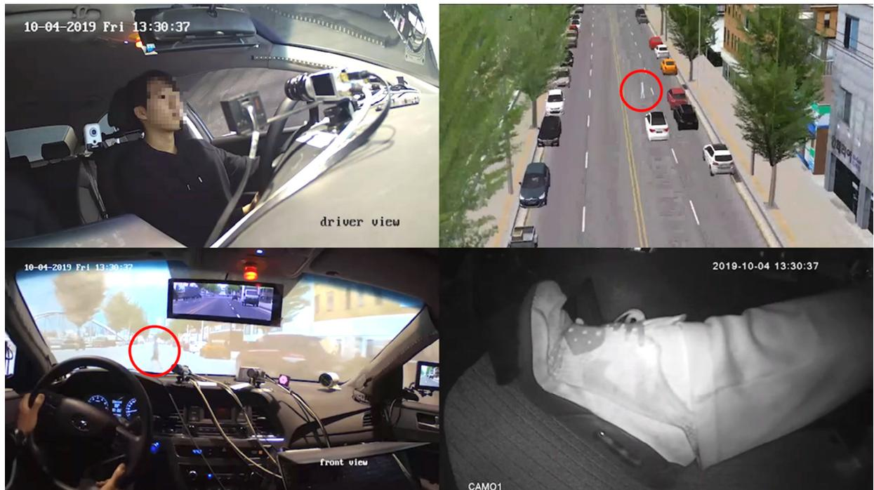
Fig. 4 Example video capture of the experiment in danger situation, subject is fully braking and steering right to evade the jaywalking pedestrian (inner red circle)
