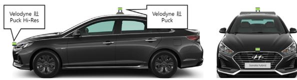
Fig. 5 Installation of LiDAR sensors on test vehicle
