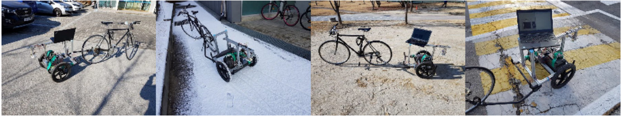
Photo. 3 Sample scenes where data sets are obtained on various road types using the experimental equipment. Collecting database using sensor module on bicycle. Asphalt, snow, earth, and painted road surfaces are listed in order
