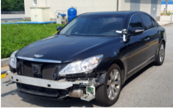
Photo. 1 Ultrasonic transmitter and receiver are installed in front of frontal tires with the ground facing
