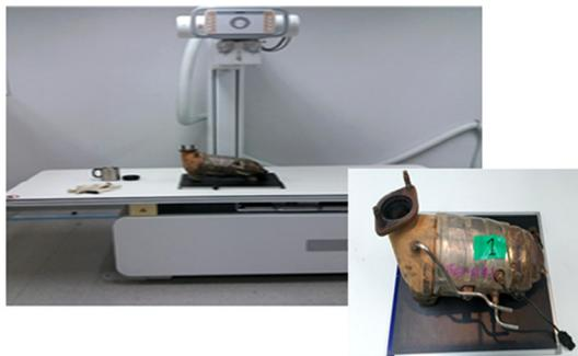
Fig. 3 The DPF removed from the vehicle in use
