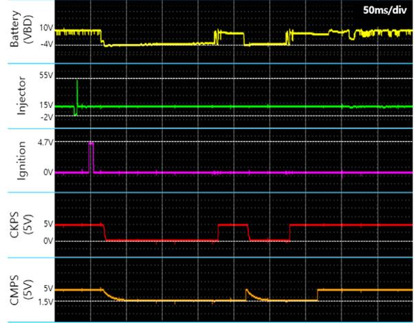
Fig. 14 Measured transient voltages at five points (VBD, CKPS 5 V, CMPS 5 V, Injector, Ignition) in the ECU immunity test setup of Fig. 11 when transient voltage is injected in power line VBD of ECU
