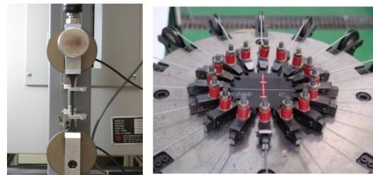
(a) Uni axial tension (b) Equi-biaxial tension
