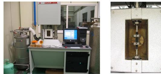
(a) Dynamic test equipment (b) Environmental chamber
