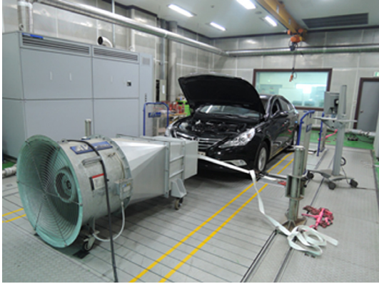
Fig. 10 Test vehicle and chassis dynamometer
