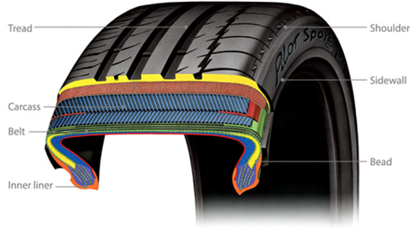
Fig. 1 Tire structure(from Steelmate Automotive)
