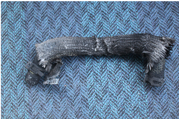
Photo. 12 Disjoined rubber hose collected by evidence
