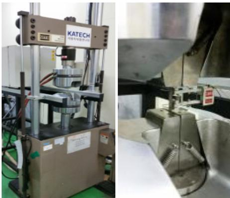
Photo. 3 Material testing system and tension test
