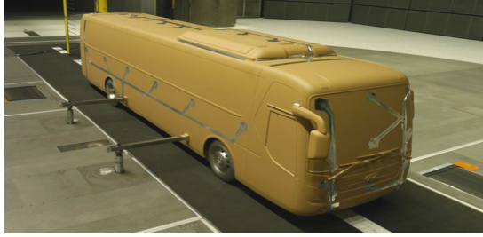
Fig. 13 1/4 scale model in the test section of wind tunnel
