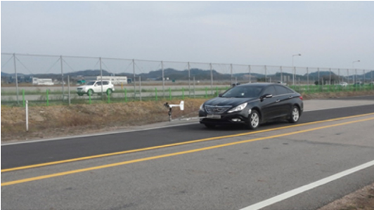
Fig. 1 Road Load measurement using onboard anemometry and coastdown techniques (SAE J2263)
