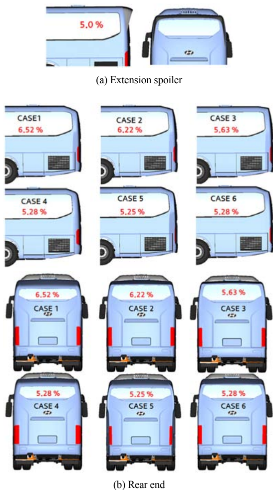
Fig. 8 Optimized design concept of spoiler and rear end
