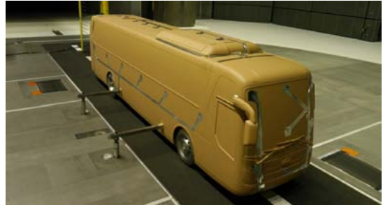
Fig. 2 Wind tunnel test of 1/4 scale model under moving ground condition
