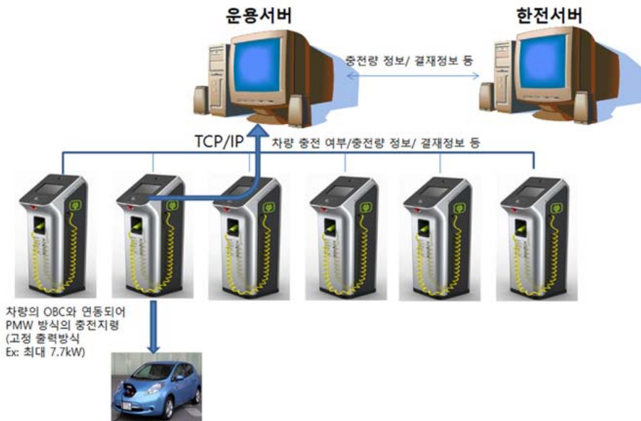
Fig. 2 Conceptual diagram of distribution switchboard for slow charger of EV able to distribute as power capacity
