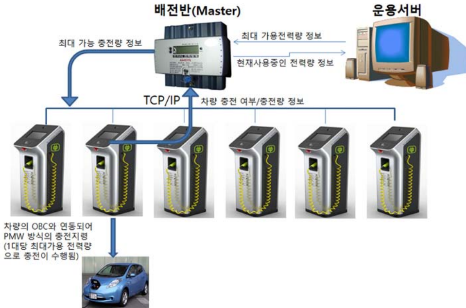
Fig. 4 Conceptual diagram of distribution switchboard for slow charger of EV able to distribute as power capacity
