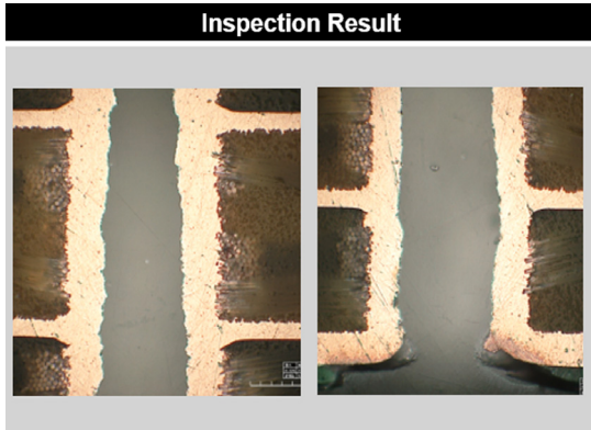
Photo. 10 PCB plated through hole inspection by microscope
