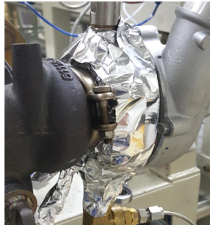
Fig. 8 Insulation of the CHRA for set up to test
