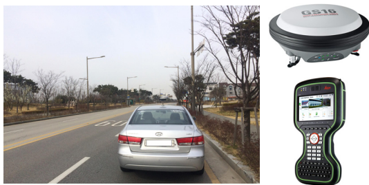
Fig. 9 Test environment(left) and rover equipment(right)
