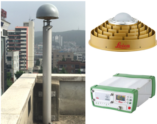
Fig. 2 MJOO GNSS permanent station(left) and GNSS equipment(right)
