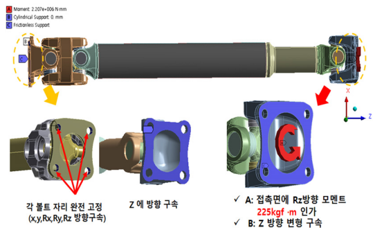
Fig. 5 Load and boundary conditions of analysis model
