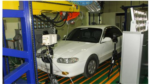
Fig. 6 Impact test of headform
