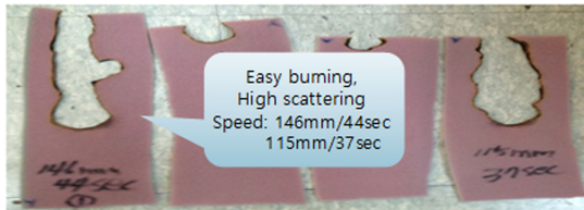
Fig. 3 Automotive standard MS-300-08 flammability test
