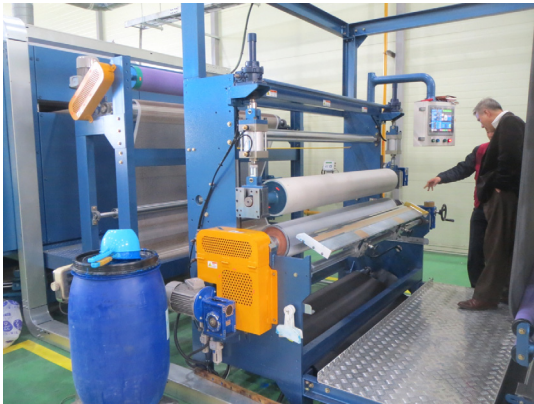
Fig. 13 Prototype of the developed coating machine
